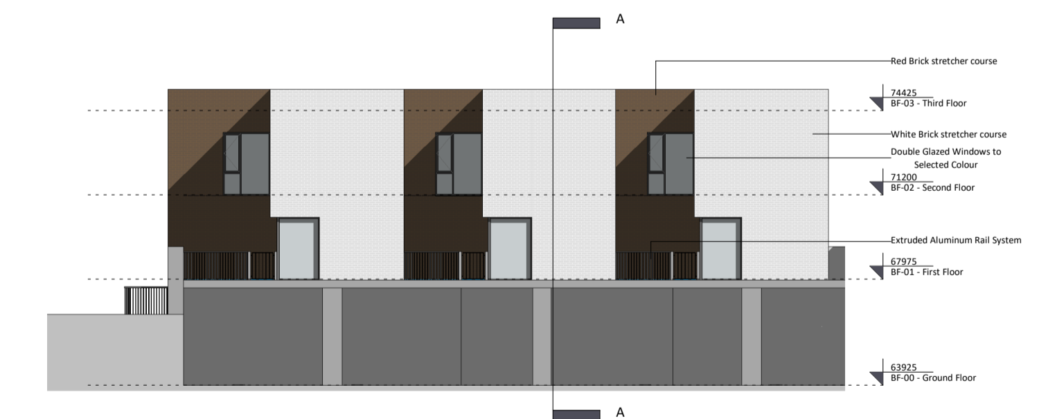
7 Block F East Elevation Duplexes 1:200
